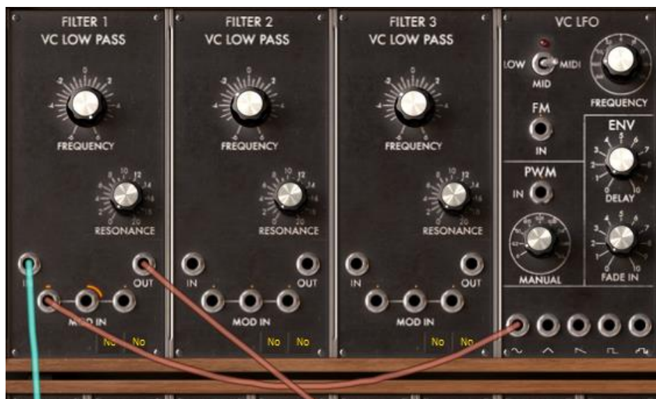
Connection of LFO to filter1
