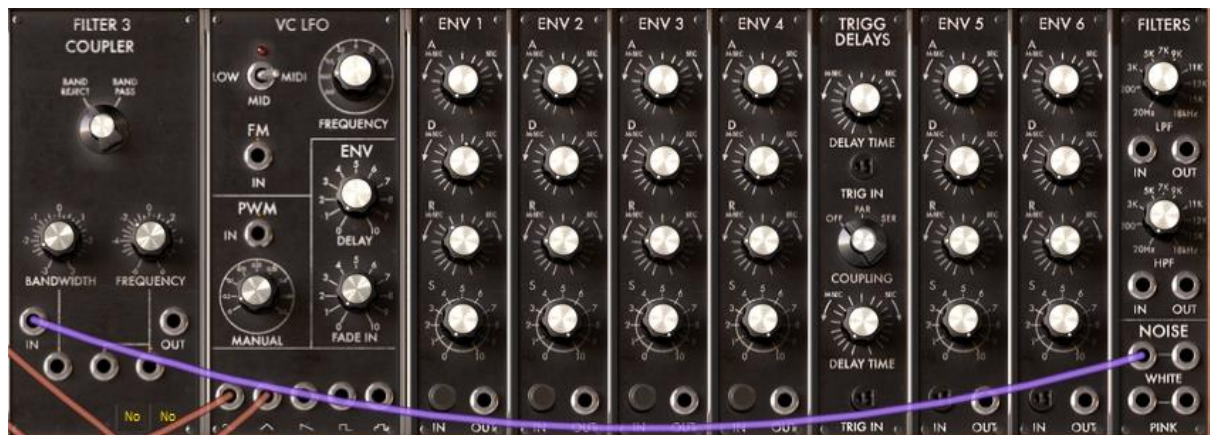
The white noise module connected to the band pass filter
