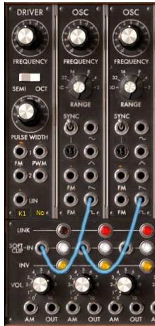
Connection of oscillators to mixer
