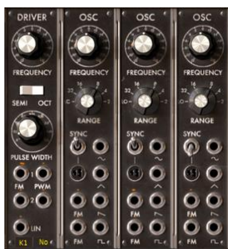
An oscillator bank: 1 “driver” and 3 “slave oscillators”
