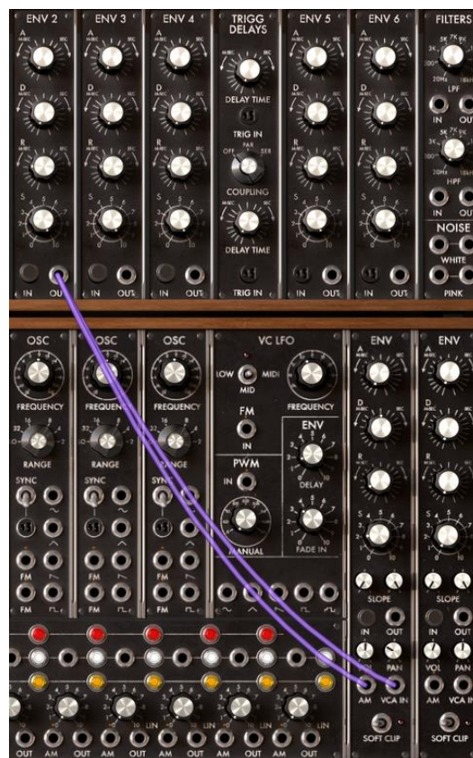
Connection of an auxiliary envelope for the output VCA
