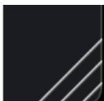
Grab and drag the diagonal lines to the right of the Macro controls to resize the Wurli V3 window. When you release the mouse, the window will snap to the closest size available in the [Resize Window \[p.51\]](#) item of the [main menu \[p.49\]](#).
